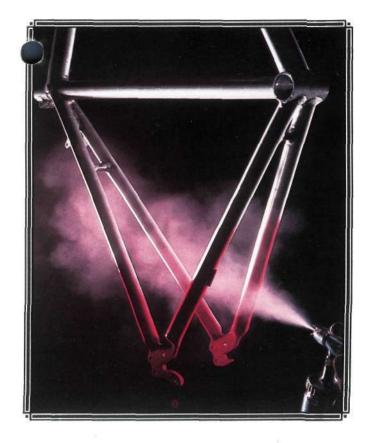
After being fully assembled and heat treated, each frame is thoroughly cleaned and given an iron phosphate coating, which inhibits corrosion and provides excellent paint adhesion. We then electrostatically apply a thick coat of Dupont Imron polyurethane enamel – the finish used by most custom frame builders – and place each frame in an oven for forced drying. The end result is a beautiful, rich, long-lasting finish that we refuse to cover up with a lot of decorations and decals.
